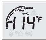
Fig. 56 Locked condition
