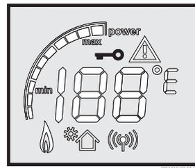
Fig. 45 Locked condition indicator (only with remote control)
