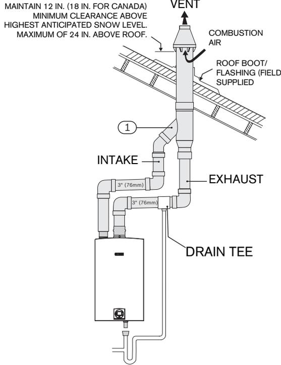
Fig. 26 Vertical venting system (sealed combustion)
