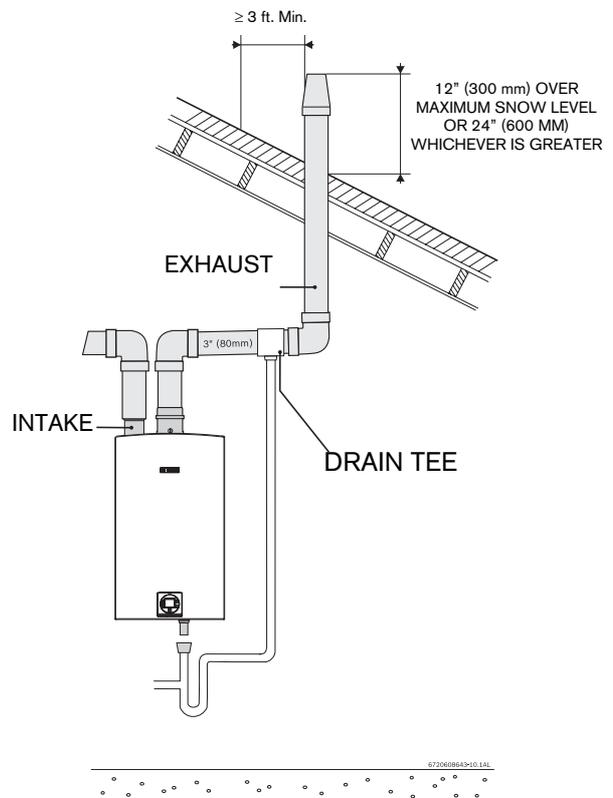
Fig. 28 Vertical venting system (room air only)
