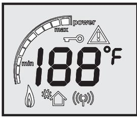
Fig. 43 Temperature indicator
