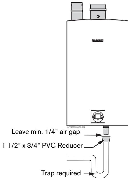
Fig. 34 Appliance drain installation
