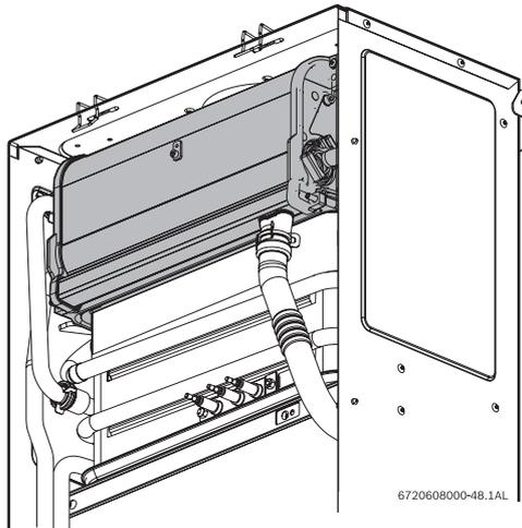
Fig. 59 Condensing heat exchanger unit
