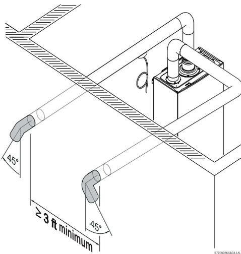
Fig. 31 Horizontal parallel venting system (sealed combustion)
