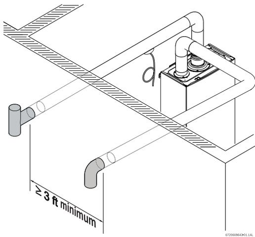
Fig. 30 Horizontal parallel venting system (sealed combustion)
