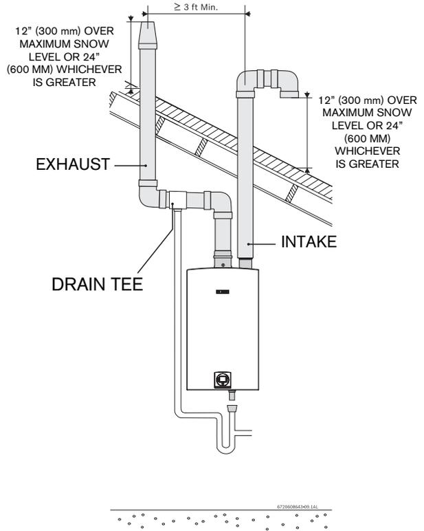
Fig. 27 Vertical parallel venting system (sealed combustion)
