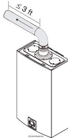
The minimum exhaust vent length is 3 feet (1 m) with one 90 degree elbow.
